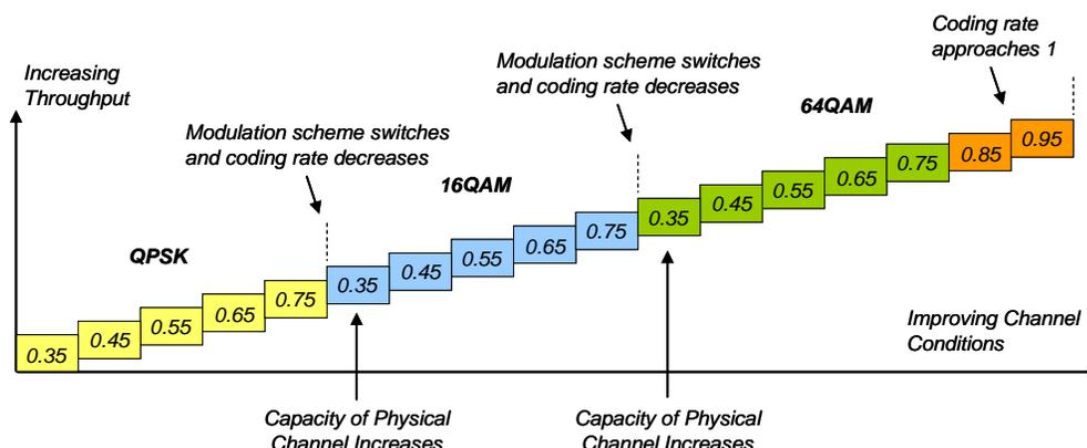
Figure 192 – Physical layer coding rate as a function of channel conditions and modulation scheme
